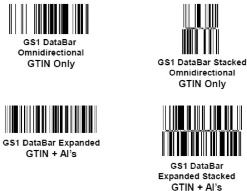
Figure 3-3. GS1 DataBar symbols used at POS
